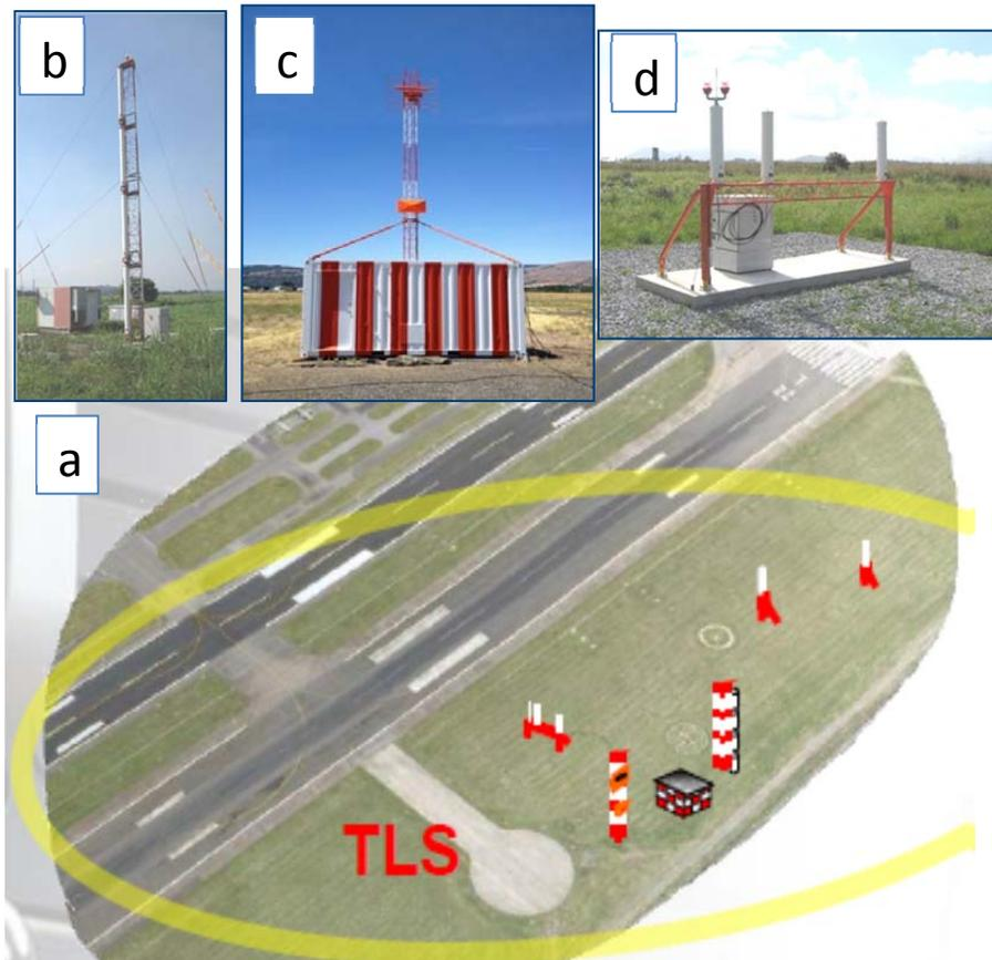
Each TLS (including antennas) would be shipped in a single 6-m-long CONEX box, which would serve as the electronic shelter. Installing the TLSs would include delivering the shelter, antenna, and generator; drilling holes for the antenna towers at four locations; installing the antennas on towers; and connecting fiber optic and power cables. The fiber optic and power cables would be buried in trenches.
