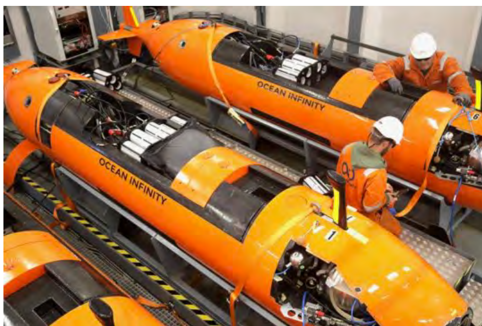
Figure 6. Ocean Infinity's Hugin Underwater Autonomous Vehicles. Two of these will be available to the Expedition.
