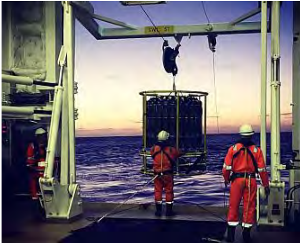
Figure 10. CTD and water sampling device being lowered through the 'environmental hangar' on the SA Agulhas II. Source: www.saeon.ac.za .
