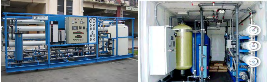
Figure 2-28 Integrated SWRO installed in a customized 20' ISO shipping container
