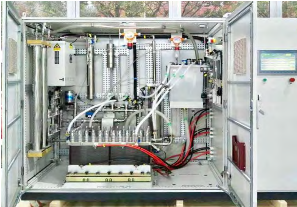
Figure 2- 41 Schematic diagram of water electrolysis hydrogen production equipment
